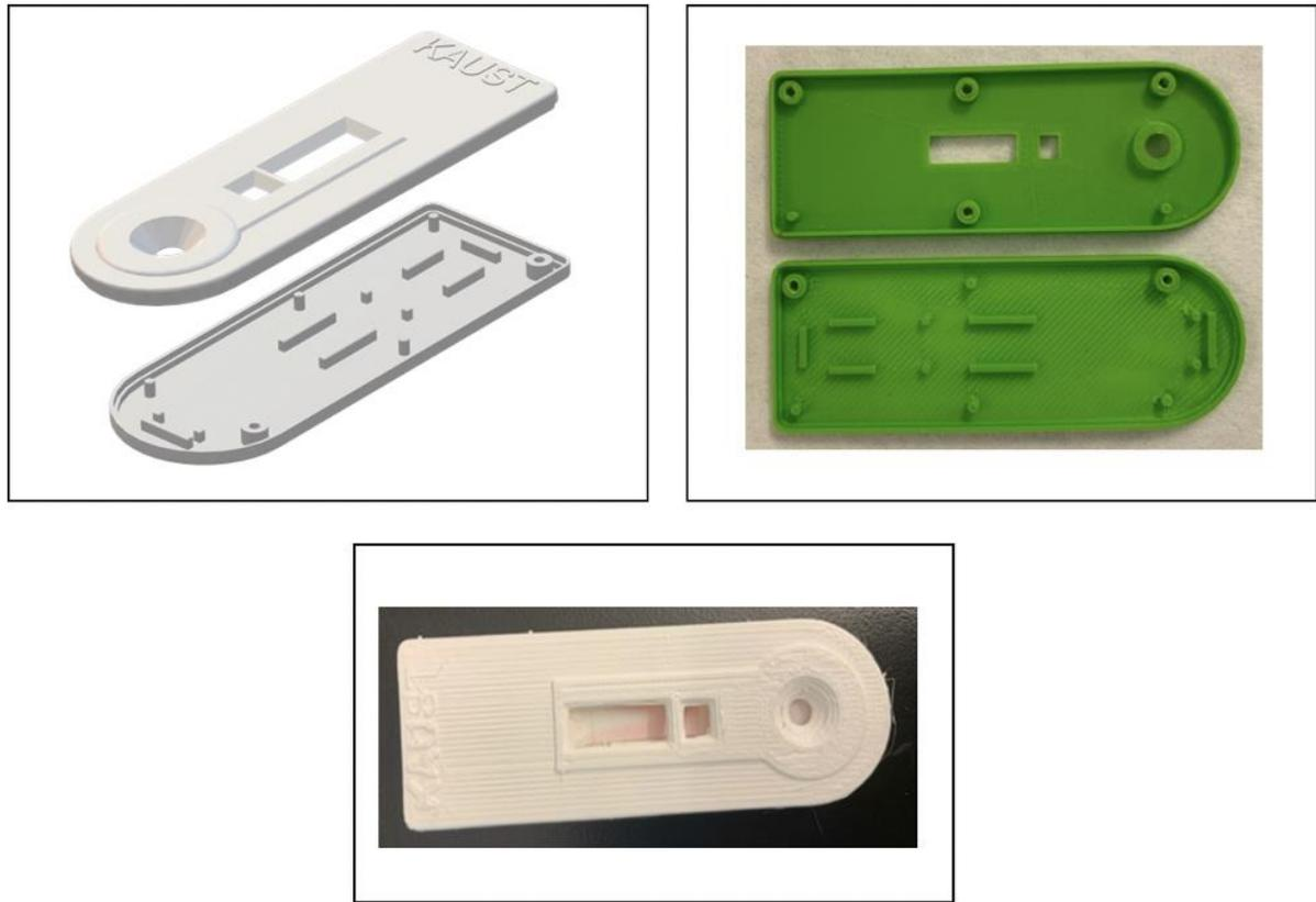
**Figure S3.** CAD of the second iteration design 3D printed housing unit using material extrusion 3D printing. 3D printed housing unit using vat photo polymerization 3D printing.
